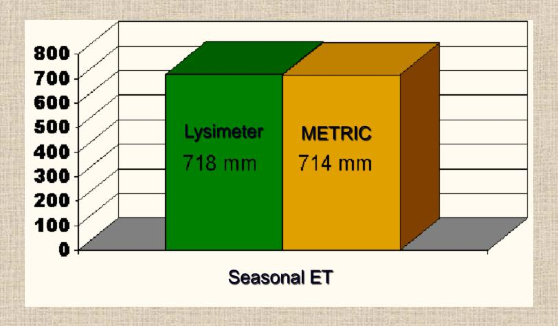
Comparison of seasonal ET as measured by lysimeter and computed by METRIC for sugar beets at the Kimberly Research Station, for April to September, 1989.
