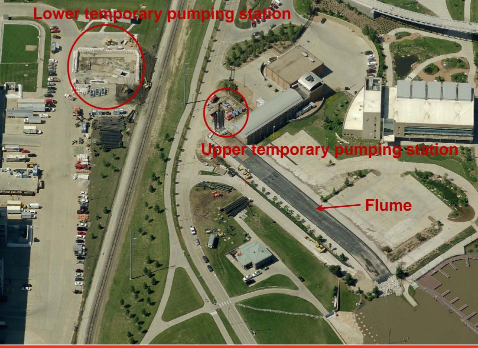
Total pumping capacity 110,000 GPM
