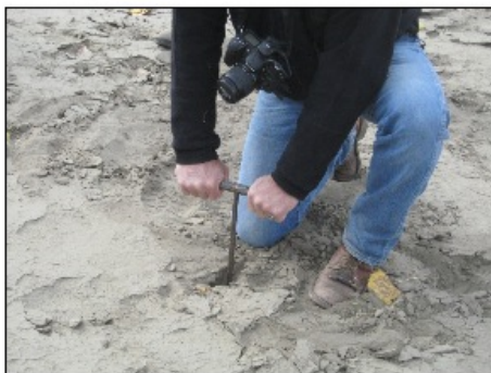
Figure 7. Four foot long sediment probe sinking into buried field.
