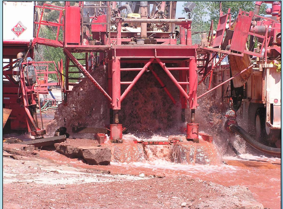
Overpressure well blowout, Park Center Well, Fremont Co.
